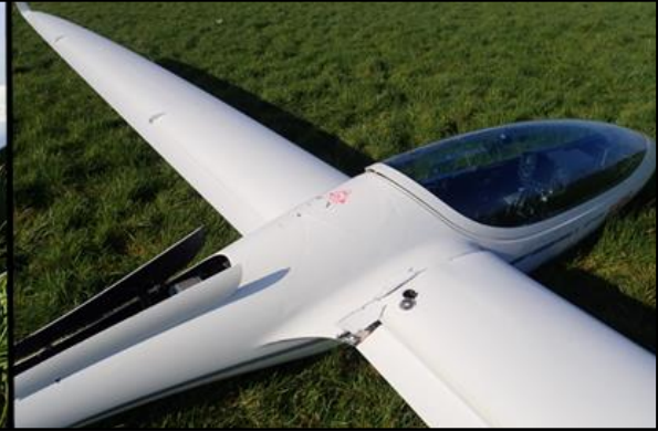
Photo No. 5: Flaperon area damage
