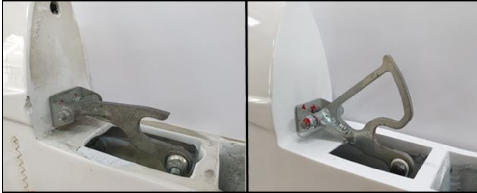
Figure No. 7: Old (left) and new (right) redesigned hook mechanism
