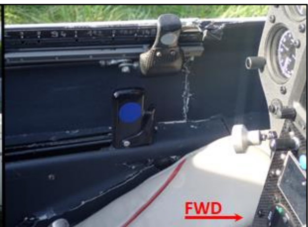
Photo No. 3: Cockpit fracture (internal)
