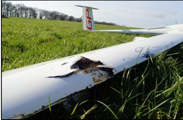
Photo No. 4: Leading edge damage
