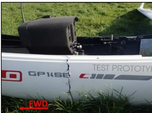
Photo No. 2: Cockpit fracture (external)
